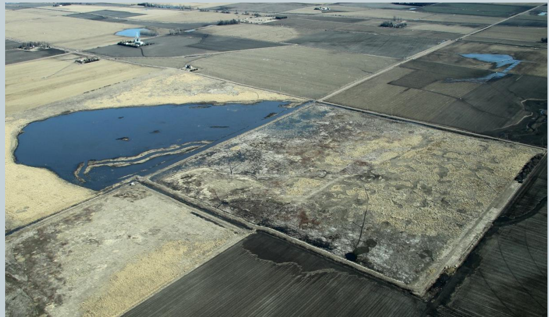
Funk Whitefront Unit at full pool, note the spoil piles are above the ponded elevation
